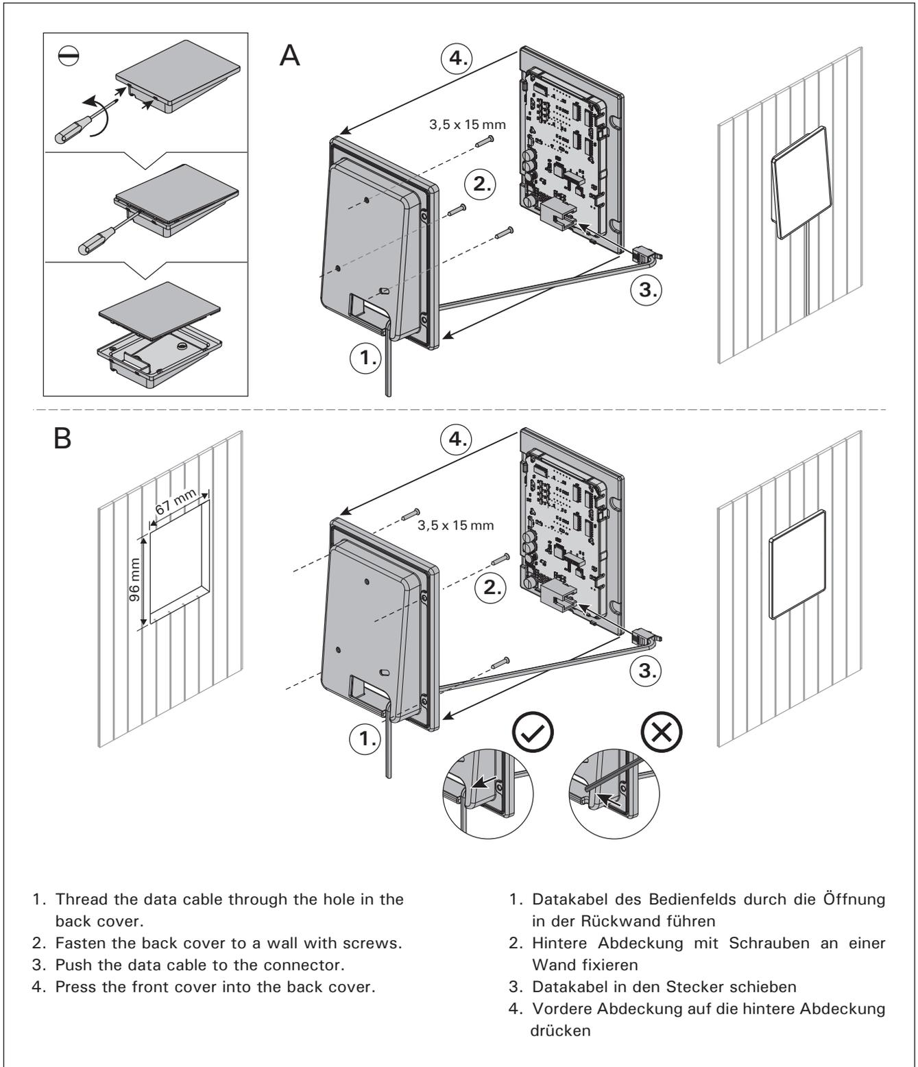
**Figure 9. Installing the control panel**
