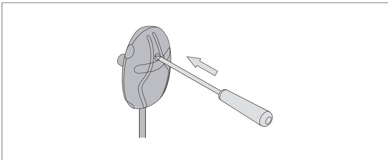
Figure 11. Reset button for overheat protector
