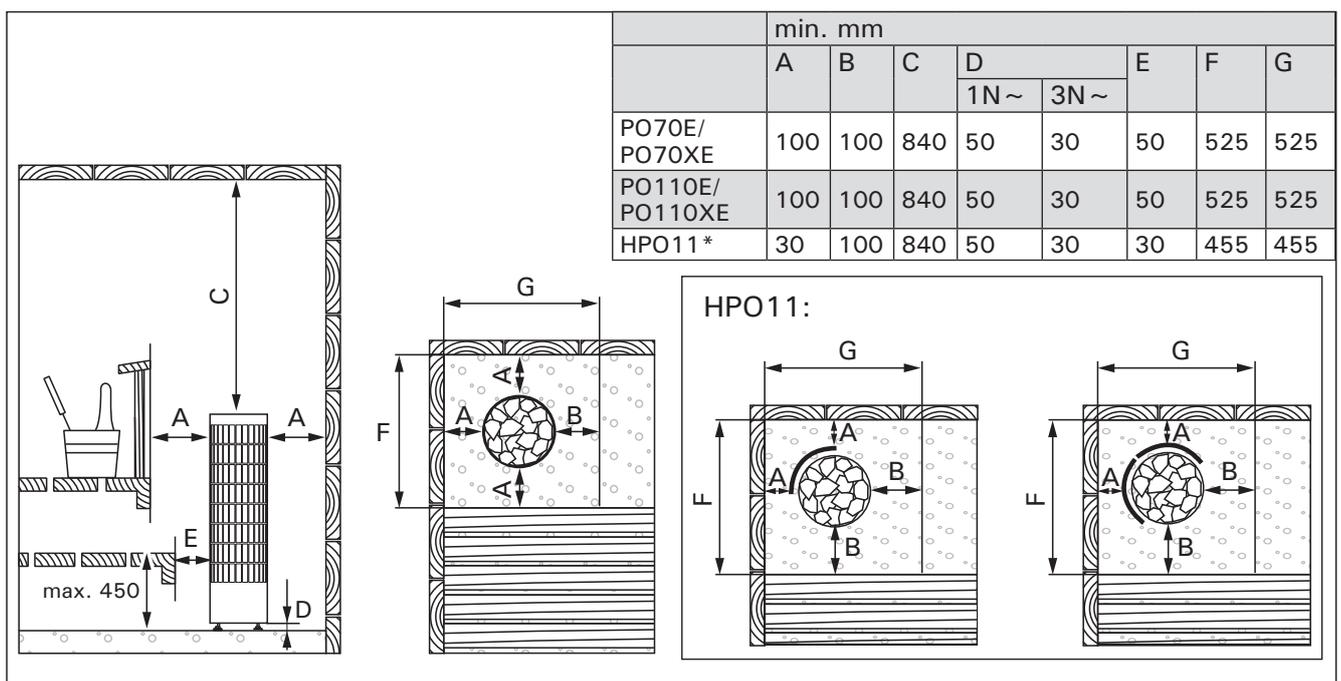
Figure 6. Safety distances (all dimensions in millimeters)
